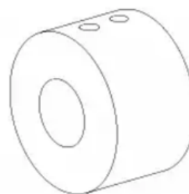
Shaft fixing method setscrew
