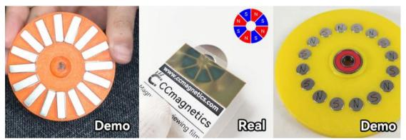
All sizes of CCmagnetics' magnetic disc couplings use sector-shaped magnets for torque transfer. These magnets maximize the use of the disc surface area, eliminating redundancy. The image above, captured using magnetic field viewing film, illustrates this point by showing the magnetic field distribution within a CCmagnetics magnetic disc coupling.
