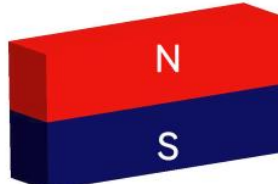
磁化长度 Magnetized Through The Width
